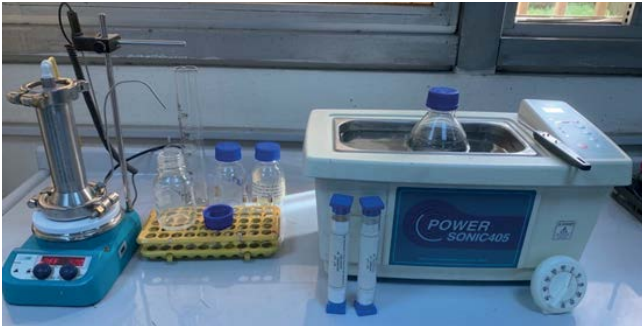
Fig. 1. Photograph of Sterlitech bench scale and a Power-Sonic 405 (5 L) ultrasonic cleaner for water treatment.
